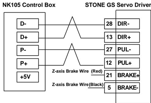
Fig. 10-9 Wiring diagram of NK105 and STONE GS servo driver
