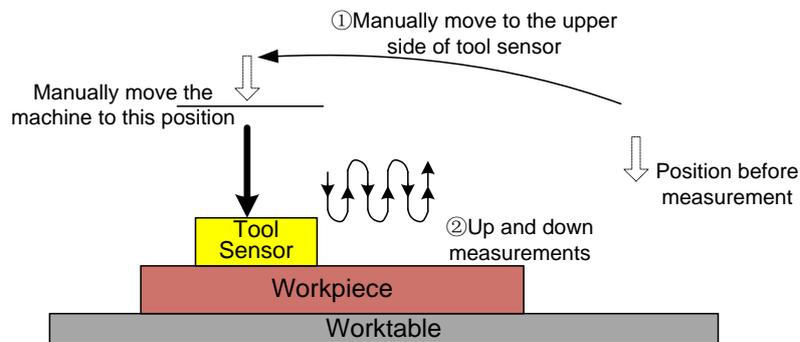
Fig. 8-1 Sketch map of moveable tool measurement
